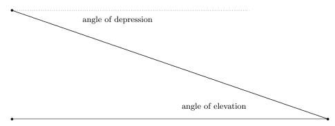
**angle of elevation**: Angle formed by a horizontal ray and a line-of-sight ray that is above the horizontal. See the diagram above. [504]
